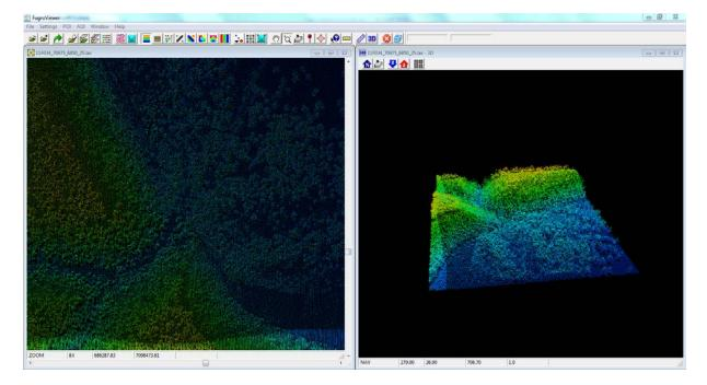
To open a .las-file, you can use the menu File->"Open LiDAR File(s)" in FugroViewer or drag and drop the file into the FugroViewer window. Also files written in text format can be opened with drag and drop. If you open a text file, you get an additional window where you must specify the format of the data. If you open a .las file, the file opens automatically.
